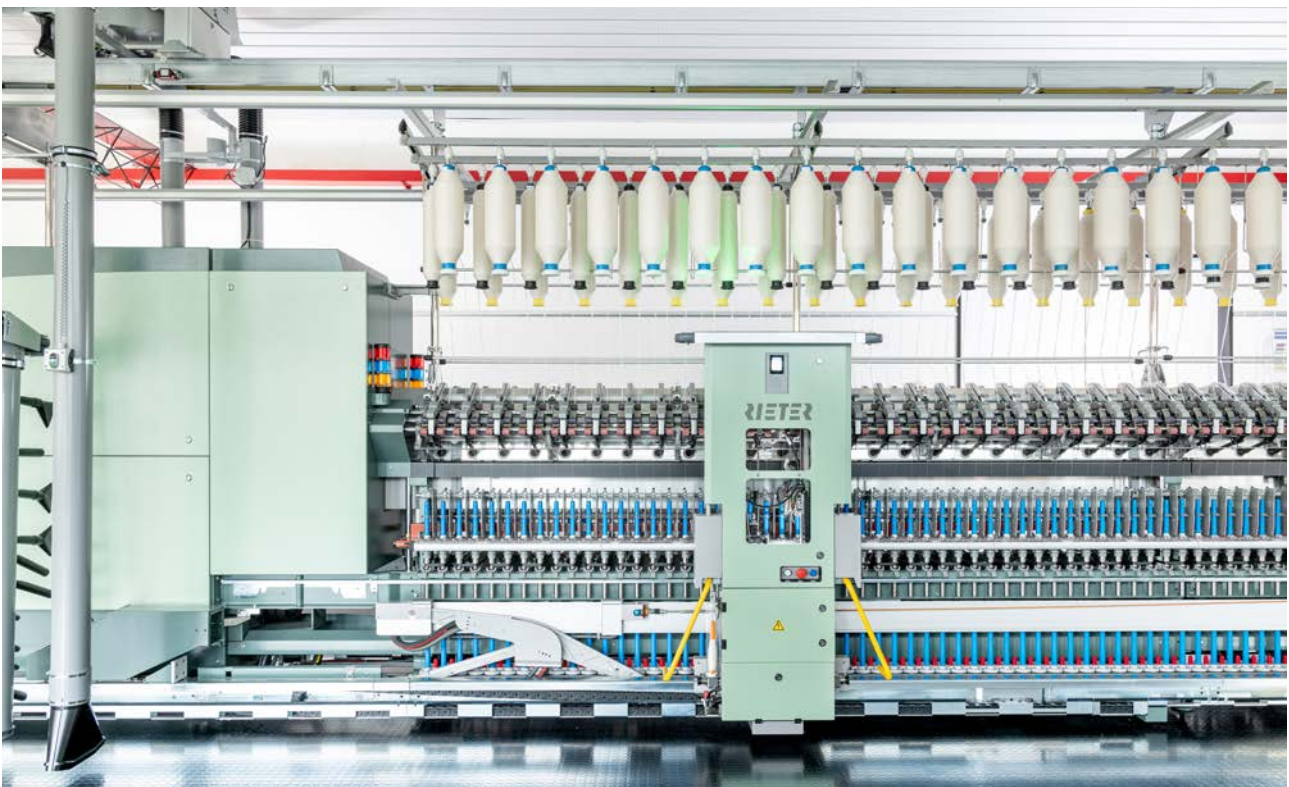
Now also available for compact-spinning machines: the ROBOSpin piecing robot
