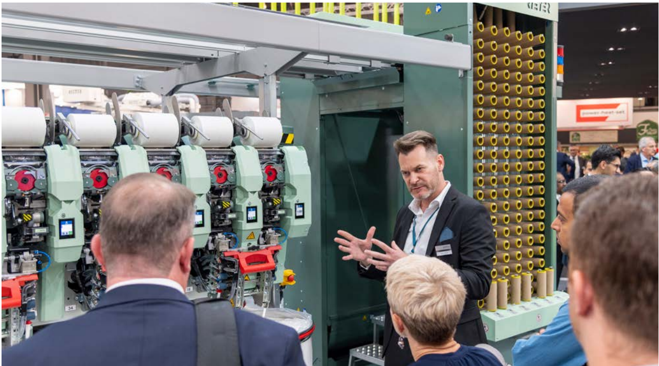
Delivery speeds up to 600 m/min: the new air-jet spinning machine J 70
